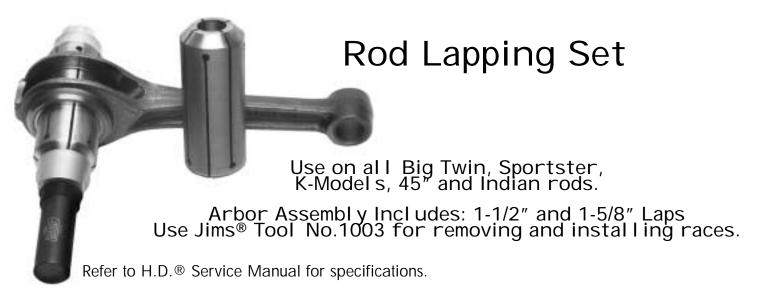
When new rods are installed, or when fitting oversize rollers, they must be lapped to fit. There are two reasons for this:
