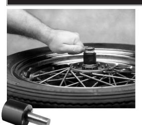
WHEEL BEARING LOCKNUT SOCKET USE ON BIG TWIN AND SPORTSTER - 1967-72
