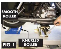
**2.** Lower the rear tire down to stand allowing the full weight of motorcycle to rest on the rotator stand tool.
