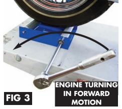
**Examples of stand use:** This is just one example of this tools usage. This stand may be used to service the primary chain adjustment, look for any tight spots on the chain. locate any loose spokes, and for cleaning front and rear tires and wheels.
