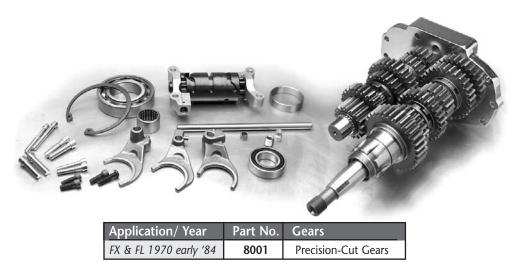
For ease of installation it is recommended to use JIMS No.8096 or 8096P 4/5 transmission cases. Before beginning the installation of this super kit transmission you should read the complete instructions and refer to the exploded parts drawing and parts list on page 3 & 4. You will need a Harley Davidson<sup>®</sup> service manual that cov-
