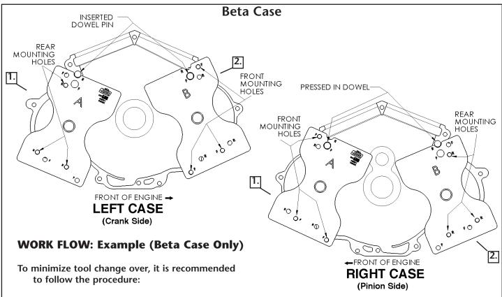
1. Install bearing using A side of plate up on the right case front. Then install bearing using A side of plateup on the left case rear bearing.
