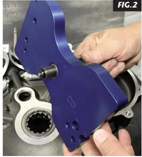
2. Screw the bearing installer pilot #5833-2 onto the screw #1024 and hand tighten, then back off 1/4 turn. See Fig. 3.
