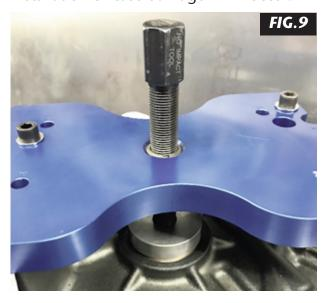
12. Remove the three  $5/16-18 \times 1-1/2"$  SHCS #1217 and remove the Balancer Bearing Installation Plate. Disassemble and store appropriately.
