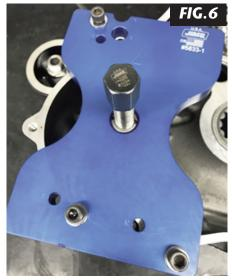
6. Align the bearing installer pilot #5833-2 with the balancer bearing bore and carefully lower the bearing installler pilot by rotating the screw #1024 clockwise until it bottoms out in the balancer bearing bore, back off 1/4 turn. DO NOT force the pilot into the bore or case damage may result. Tighten the three 5/16-18 x 1-1/2" SHCS #1217 until tight with an Allen key. See Fig. 7.
