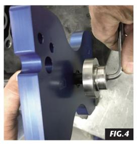
**4.** Place lubricant between the bearing installer pilot #5833-2 and the Oil-Lite bearing/bushing #5833-3. Lubricate the bottom face of the Oil-Lite bearing/bushing as shown in **Fig. 5.** Lubricate the bearing bore with Sunnen Assembly lube or similar.
