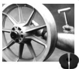
1. Refer to H.D.® service manual for specifications. Use to remove and install bearing cups in cast wheels (Use with JIMS tool handle #33416-80).
