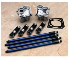
These tappet blocks supersede lifter block No.'s 18603-80A, 18610-76A and tappet No.'s 18522-53A. Fits Shovel Big Twins 1966 through 1984. Use 1/4"-20 screws, JIMS® No.1205, from late 1976 through 1984. Use 1/4"-24 screws, JIMS® No.2406, from 1966 through early 1976. These blocks are designed to accommodate a gross valve lift of .550" at the valves, leaving a clearance of .035" roller to block freeplay (Please note, if using a cam with a higher lift, a simple modification is all that is needed).
