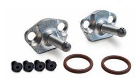
JIMS Twin Cam Piston Oiling Jets are designed with an additional .150" clearance compared to stock OEM jets. For use on longer stroked engines, always check clearances during assembly. Install piston oiling jets per H-D® or Clymer Service Manual.
